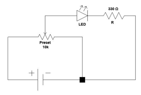
After the circuit is complete, rotate the preset.
