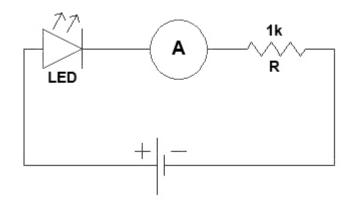
An Ammeter is a device that measures current and is always connected in series with the circuit. It is denoted by symbol 'A'. We can use a multimeter in ammeter mode.
