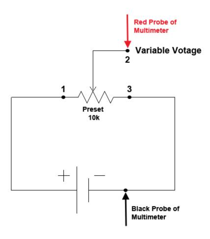
Terminal 1 of preset is given Vcc (positive) and terminal 3 is grounded (negative). Output is taken from terminal 2. Say, your preset is of 10k  $\Omega$ . So, output from terminal 2 is a variable voltage source. We can think of a voltage diver as a variable battery, which can provide voltage varying from zero to a rated value (maximum).
